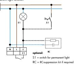
Standard mode with 1-channel motion detector
