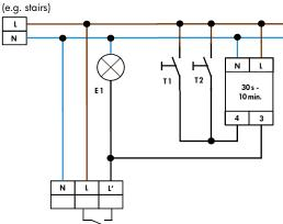
Standard mode with 1-channel motion detector with NC pushbutton
