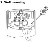
Mount the plug-in socket with two screws and the enclosed seal rings on a firm base. (Pay attention to inserting of the connection cable, see point 3)
