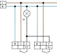
Standard mode with 1-channel motion detector with permanent light function
