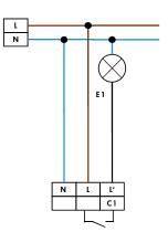
Parallel connection with 1-channel motion detectors max. 2 parallel
