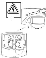
1) Caution: have all work involving the 230 V mains supply carried out by a qualified electrician! Before starting disconnect the mains! Please be aware that the LUXOMAT<sup>®</sup> LC-Click-N 140/200 is not suitable as an intrusion detector, since it is not equipped with a tamper contact. 2) Socket base corner mounting
